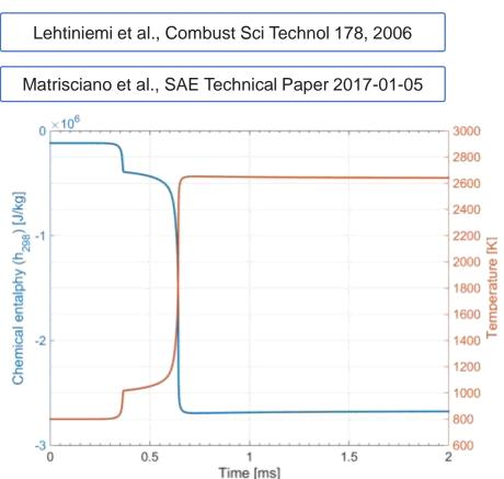
Chemical enthalpy and temperature as a function of time for a constant pressure calculation at 10 bar and 750 K for an n-heptane/ air mixture at  $\phi$ =1.
