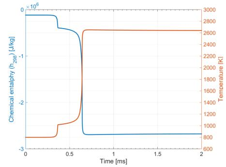
Chemical enthalpy and temperature as a function of time for a constant pressure calculation at 10 bar and 750 K for an n-heptane/ air mixture at  $\phi=1$ .
