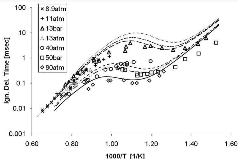
Figure 3: Ignition delay time for n-decane/air mixture at  $\phi=1.0$ ,  $p = 8.9$  atm [9], 11 atm, 40 atm [7], 13 bar, 50 bar [6], 13 atm, 80 atm [8].
