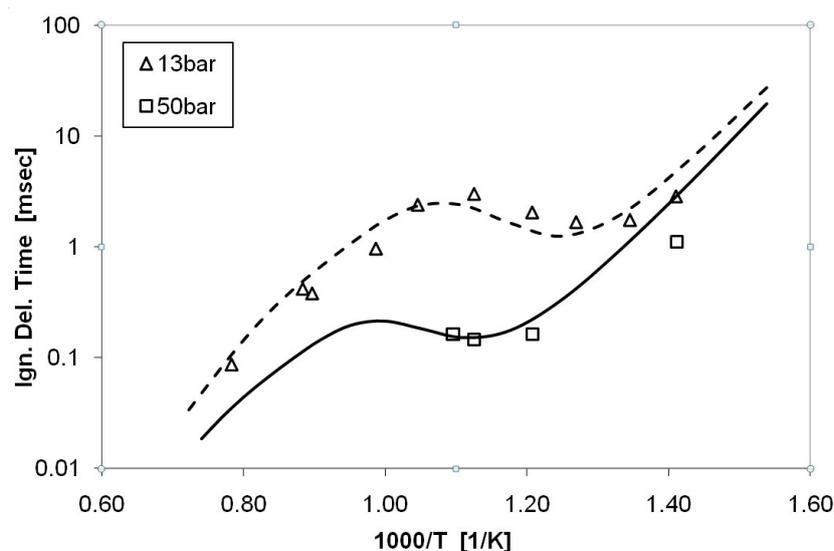
Figure 4: Ignition delay time for n-decane/air mixture at  $\phi=2.0$ ,  $p=13$  bar, 50 bar [6].
