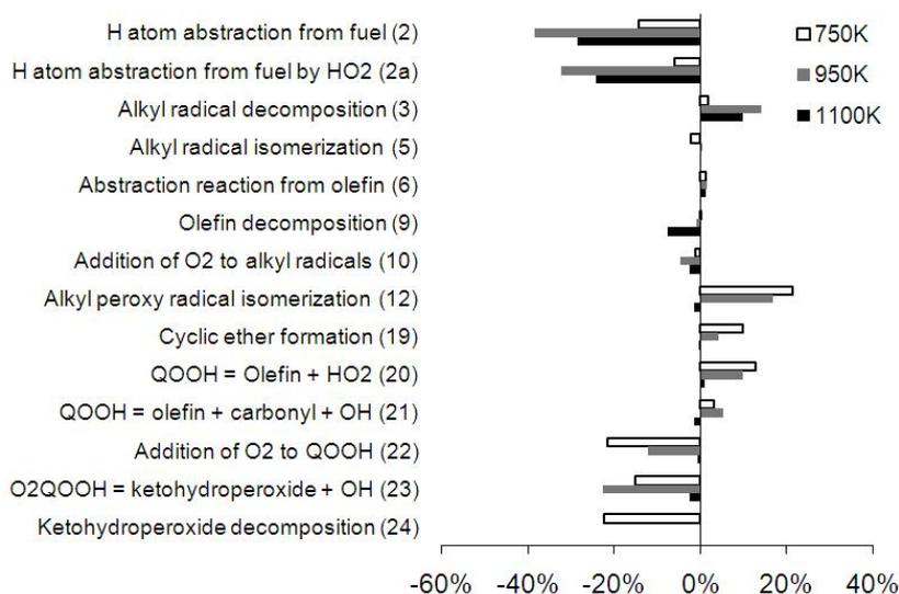
Figure 5: Sensitivity coefficients for ignition delay times for n-decane/air mixtures at three different temperatures ( $\phi = 1.0$ ,  $p = 13.5\text{bar}$ ).
