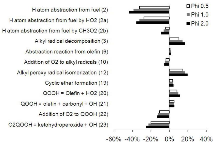
Figure 6: Sensitivity coefficients for ignition delay times for n-decane/air mixture at three different fuel air equivalence ratios ( $p = 13.5\text{bar}$ ,  $T = 950\text{K}$ ).
