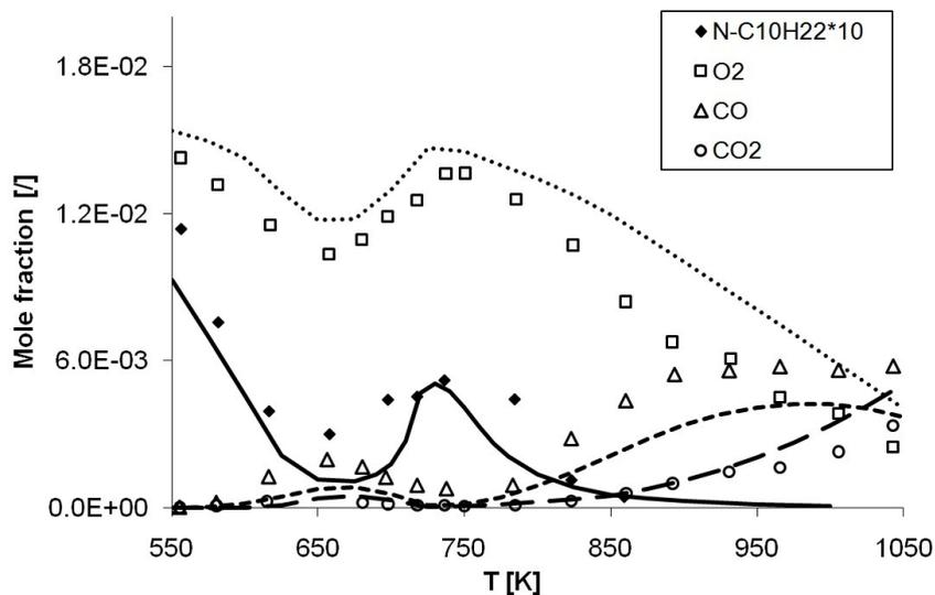
Figure 1: Concentrations of n-Decane, O<sub>2</sub>, CO and CO<sub>2</sub> in a Jet Stirred Reactor at p=10 bar,  $\phi=1.0$ , 0.1% fuel and  $\tau=1$  sec [10].
