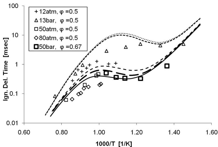
Figure 2: Ignition delay time for n-decane/air mixture at 12 atm, 50 atm [7], 13 bar, 50 bar [6], 80 atm [8]
