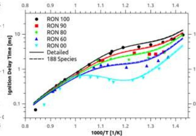
Measured ignition delay time of iso-octane/n-heptane mixtures at  $40 \pm 2$  bar,  $\phi = 1$  from Fieweger et al. [11]. Simulation for the detailed and reduced reaction scheme using upper pressure limit.
