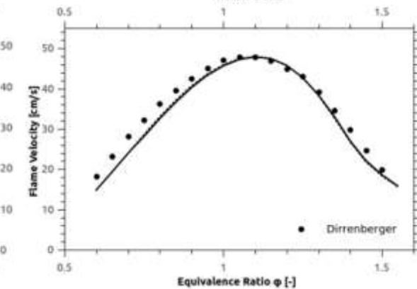
Laminar flame speeds at 1 atm and 358 K with air as oxidizer for a mixture of 11.65% n-heptane, 36.47% iso-octane, 36.88% toluene and 15.0% ethanol (liquid volume fraction). Experimental data from Dirrenberger et al. Solid line: detailed reaction scheme; Dashed line: reduced scheme.
